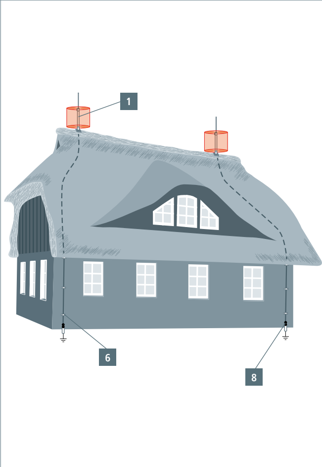
Installation of the HVI Conductor to protect a building with a thatched roof
